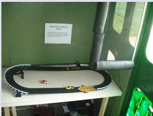
*A display that uses solar panels to power slot racing cars.*
